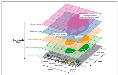
Figure 1: Graphical representation of the SGAM framework as shown in Bruinenberg et al (2012).
