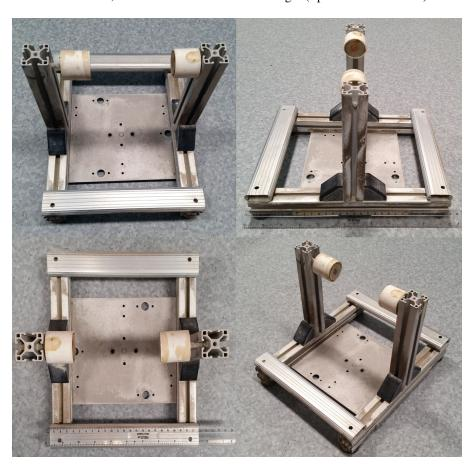
Figure S1: Motor frame used inside water tank
