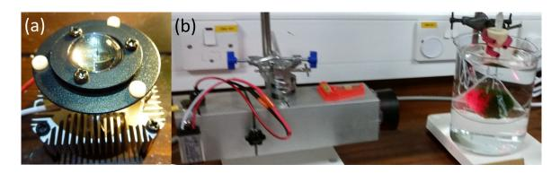
Figure S3: Bespoke lamp (a) LED array and lens on heatsink (b) narrow (4 degree) light beam
