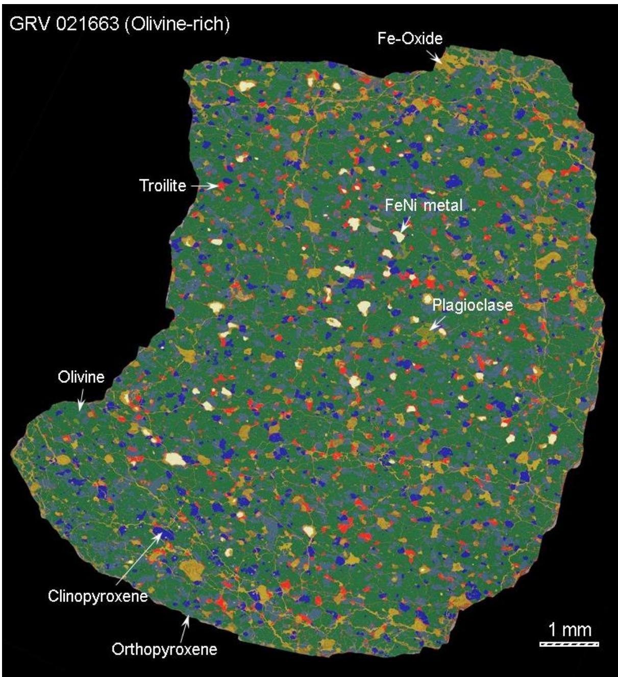
Figure A5. Elemental composite map of the coarse-grained olivine-rich texture GRV 021663
