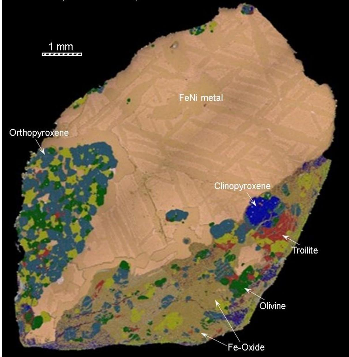
Figure A6. Elemental composite map of coarse-grained metal-rich texture NWA 4024
