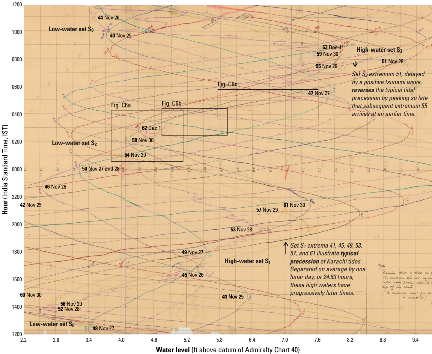
Figure C5 Scanned marigram between 2.2 and 9.7 ft on the water-level axis, showing areas of detail in Figure C6 and successive delay of high waters and low waters within lunar-day groups
